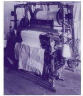
The loom temple, patented by Ebenezer's father, Ira, revolutionized the weaving process. By holding the fabric taut, the temple greatly reduced the number of hours required to manufacture cloth. Mechanized weaving led to a reduction in the cost of cloth, so that many people today own many more clothes than did their ancestors.
